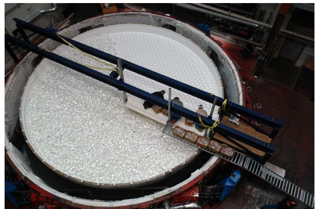
20 tons of glass being loaded into the GMT mirror furnace mould. Image credit: GMT0 Corporation
